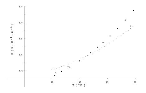
FIG.1. Thermal conductivity vs. temperature obtained by the methods: ..... inverse .... standard steady state .... standard Van –Rinsum
