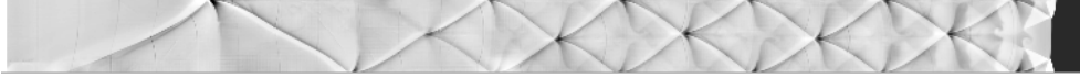
FIGURE 5.2. Time history of released chemical energy at t = 260\ \mu\text{s} . Regular detonation-cells with a width of \approx 5.3\text{ cm} are visible.
