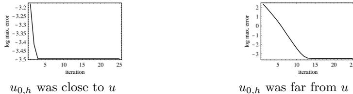
FIG. 5.4. Logarithms of  $L_\infty(\Omega)$ -errors for  $u_{k,h}$  versus iterations
