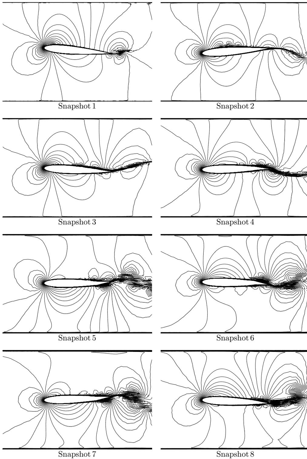
FIG. 4.2. *The velocity isolines for several time instants*
