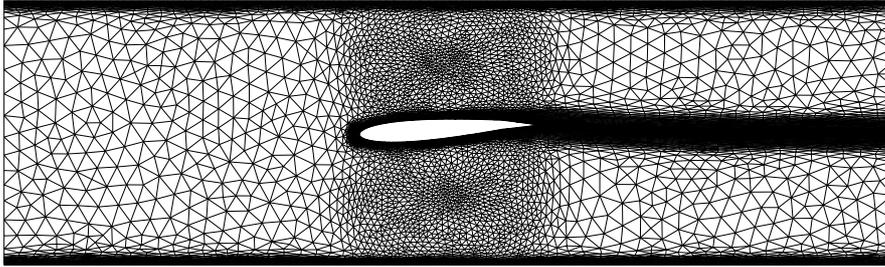
FIG. 4.1. Anisotropically adapted mesh for NACA 0012 airfoil inserted into a wind tunnel
