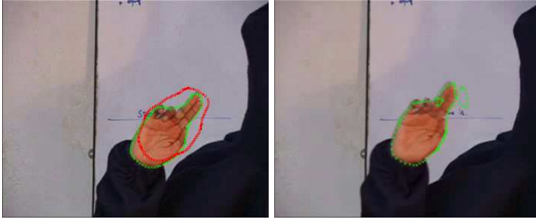
FIGURE 12. Illustration of curve degeneration. Left: The initial curve in red. Right: Bunching of points (in red) starts due to target motion leading to a loop formation.
