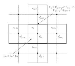
Figure 1: A description of a finite volume  $v_{ij}$  defined on the dual mesh. Here  $\Omega_{ij}$  is its interior,  $\Gamma_{ij}$  its boundary consisting of linear segments  $\Gamma_{ij,i\pm 1j}, \Gamma_{ij,ij\pm 1}$ .
