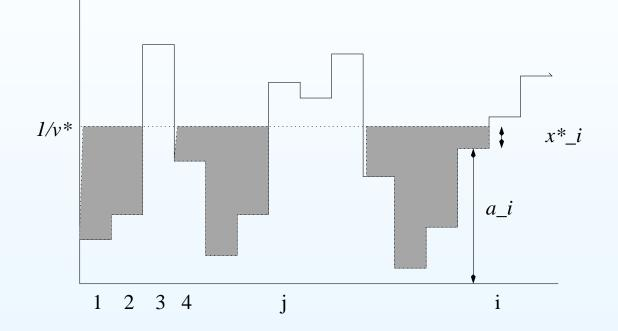
"Water filling" method: The height of each patch is given by  $\alpha_i$ . The region is flooded to a level  $1/v^*$  which uses a total quantity of water equal to one. The height of the water above each patch is the optimal value of  $x_i^*$ .
