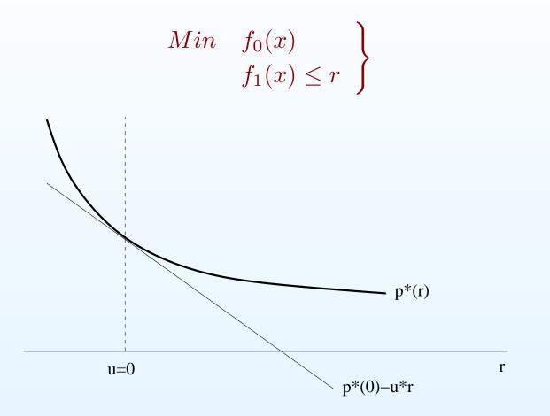
The optimal value  $p^*(r)$  of the perturbed convex problem with one constraint  $f_1(x) \le r$  is a convex function of r. Affine function  $p^*(0) - u^*r$  is the lower bound on  $p^*(r)$ .
