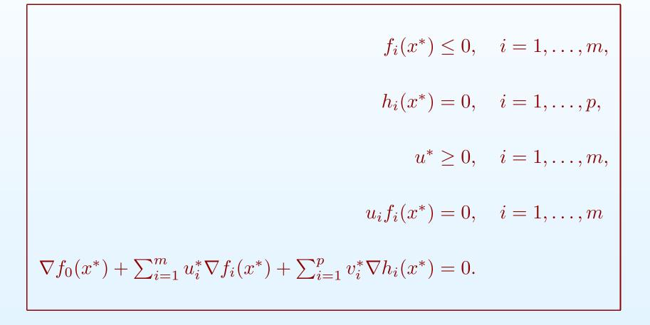
If  $x^*$  is optimal for (P) and  $(u^*, v^*)$  is optimal for (D) and strong duality property  $p^* = d^*$  holds, then
